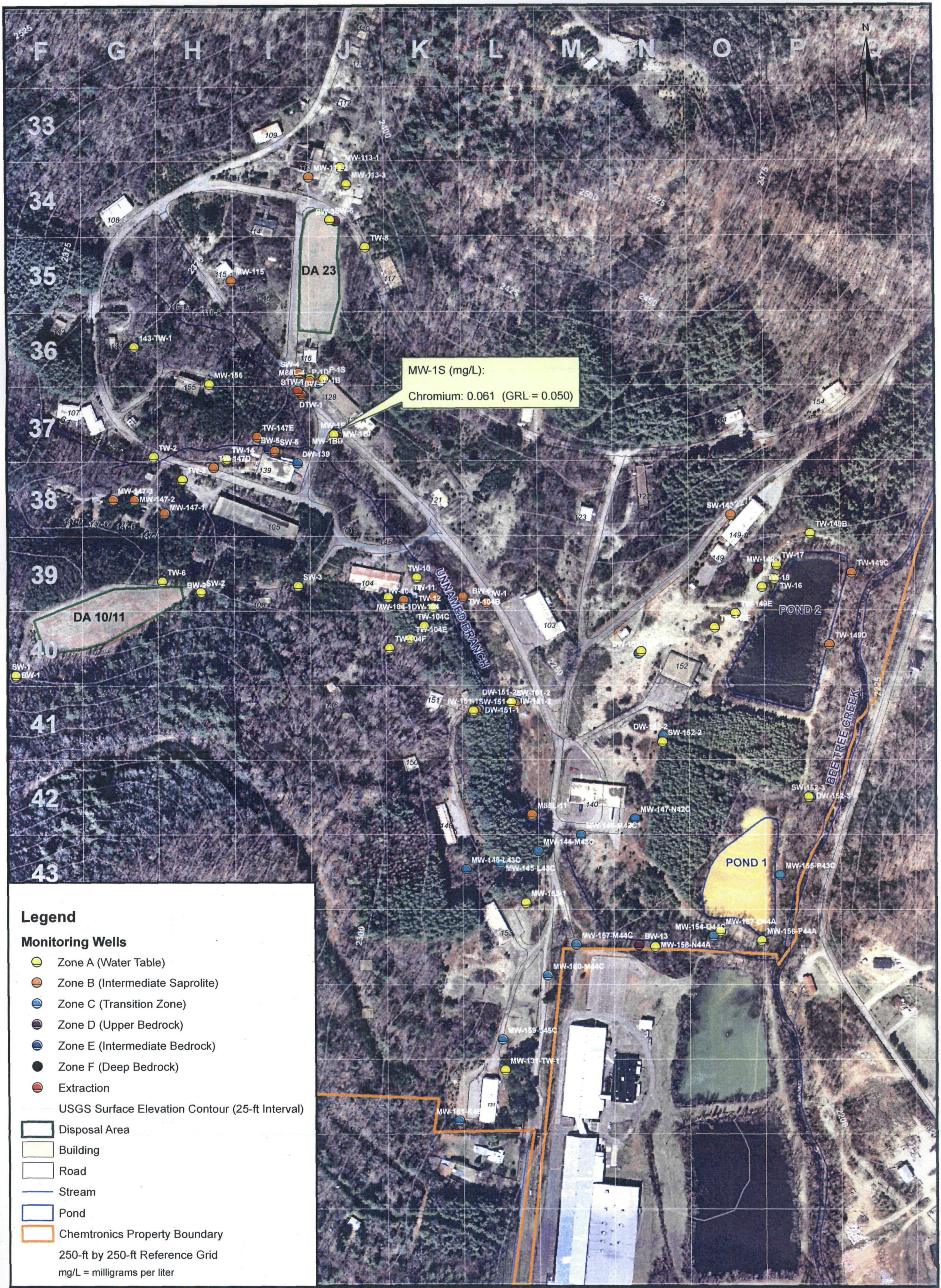
FRONT VALLEY METALS EXCEEDING THE GROUNDWATER REMEDIATION LEVEL (GRL) IN CERCLA COMPLIANCE WELLS OCTOBER 2001
